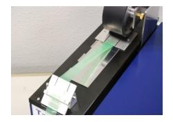
Sample installation jig conforms to JIS Z 0237(2009)
