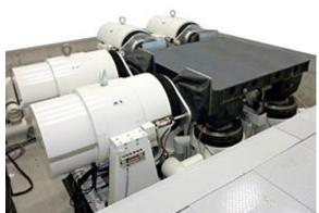
At least 6 vibration shakers are located in 3D space with integrated control and can create 6 degrees of freedom motion (3 translation degrees of freedom and 3 rotating degrees).
