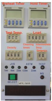
Thumbwheel switches type test condition input panel
