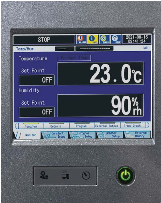
The console includes the P-300 programmer, USB port, product temperature protector, and chamber light.
