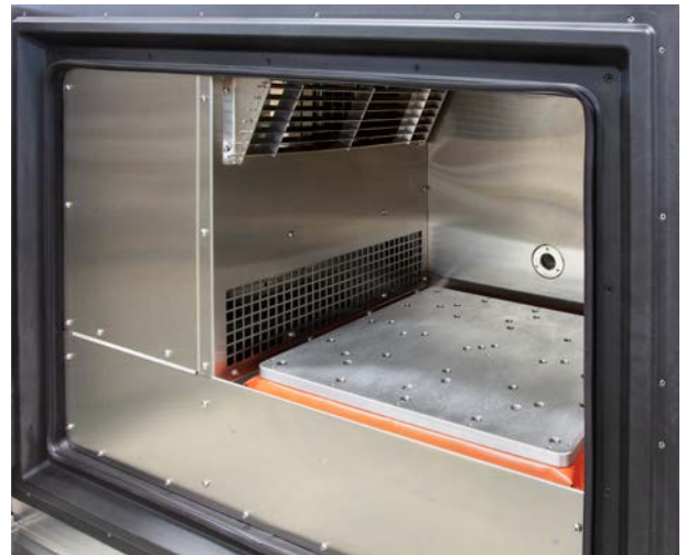
EQZ4 interior with 18" x 18" repetitive shock table
