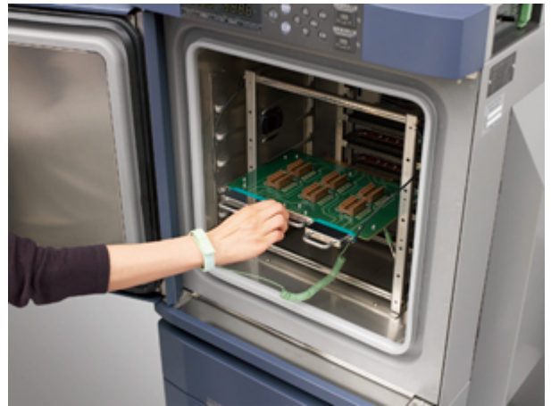
DUT board with short connector (test area)
