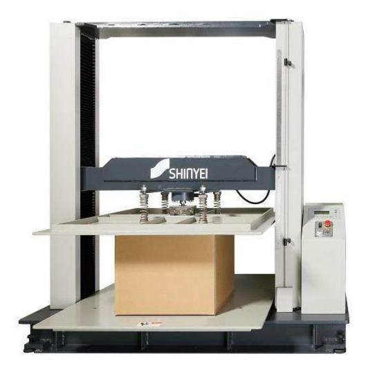
This machine is used to evaluate a compressive strength of packaging container. This test will be contributed to improve your packaging and control a quality to prevent the damage in an actual stage environment
