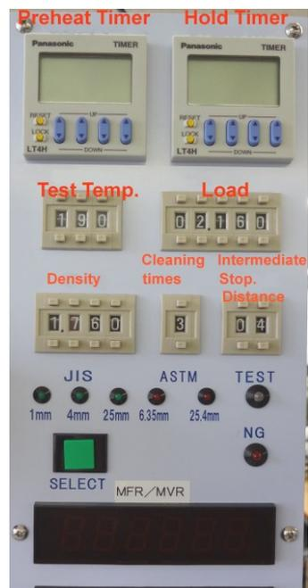
Thumbwheel switches type test condition input panel
