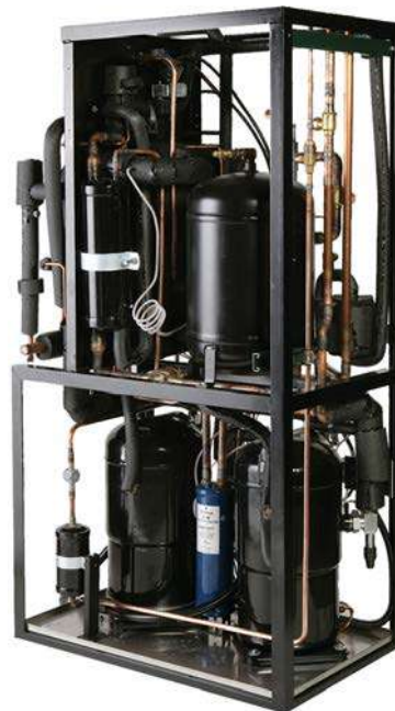
Advanced refrigeration design is especially compact for high performance test chambers.
