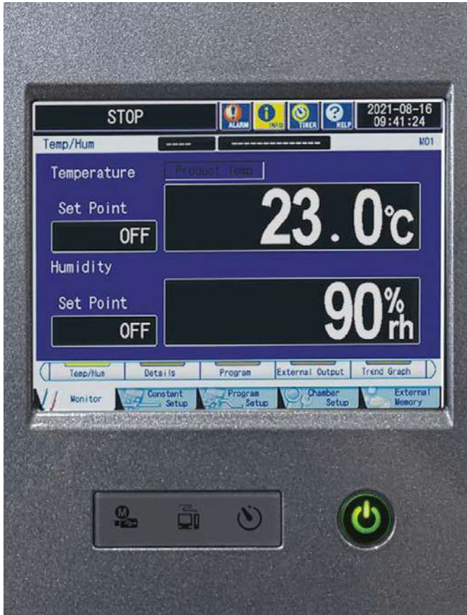
The door-mounted console includes the P-300 programmer, USB port, product temperature protector, and chamber light (option).
