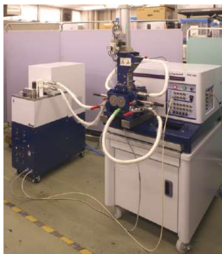
(Banbury type mixer model BR250 mixer with oil circulation bath Note: Base unit shown is old generation model)
